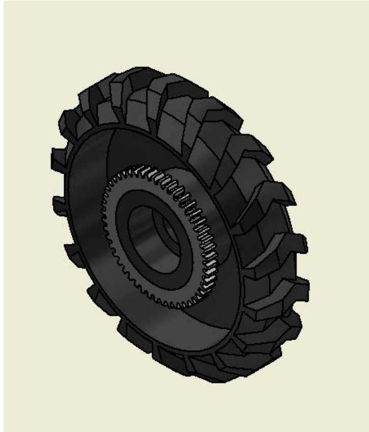
Figure 5-10: Spur gear attached inside the wheel
